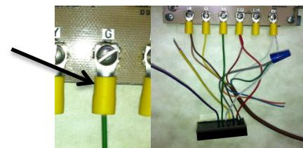
Add the **Yellow** wire of the HVAC-CHIP to the existing wire at the "Y" terminal. After the connection is complete, there should be 2 wires connected to this Y terminal.
