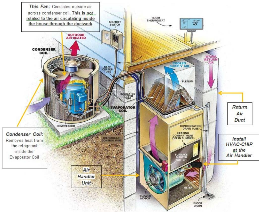
**INSTALL THE HVAC-CHIP ON THE 24 VOLTS SECTION OF THE AIR-HANDLER UNIT. SEE LOWER RIGHT CORNER OF PICTURE ABOVE**
