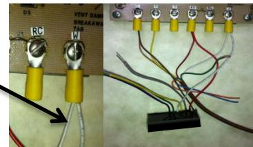
Use a wire nut, connect the **Green** wire (previously disconnected in step A) to the **Gray** wire of the HVAC-CHIP. *This means that the HVAC-Chip Gray wire is now directly connected to the thermostat's green terminal.*
