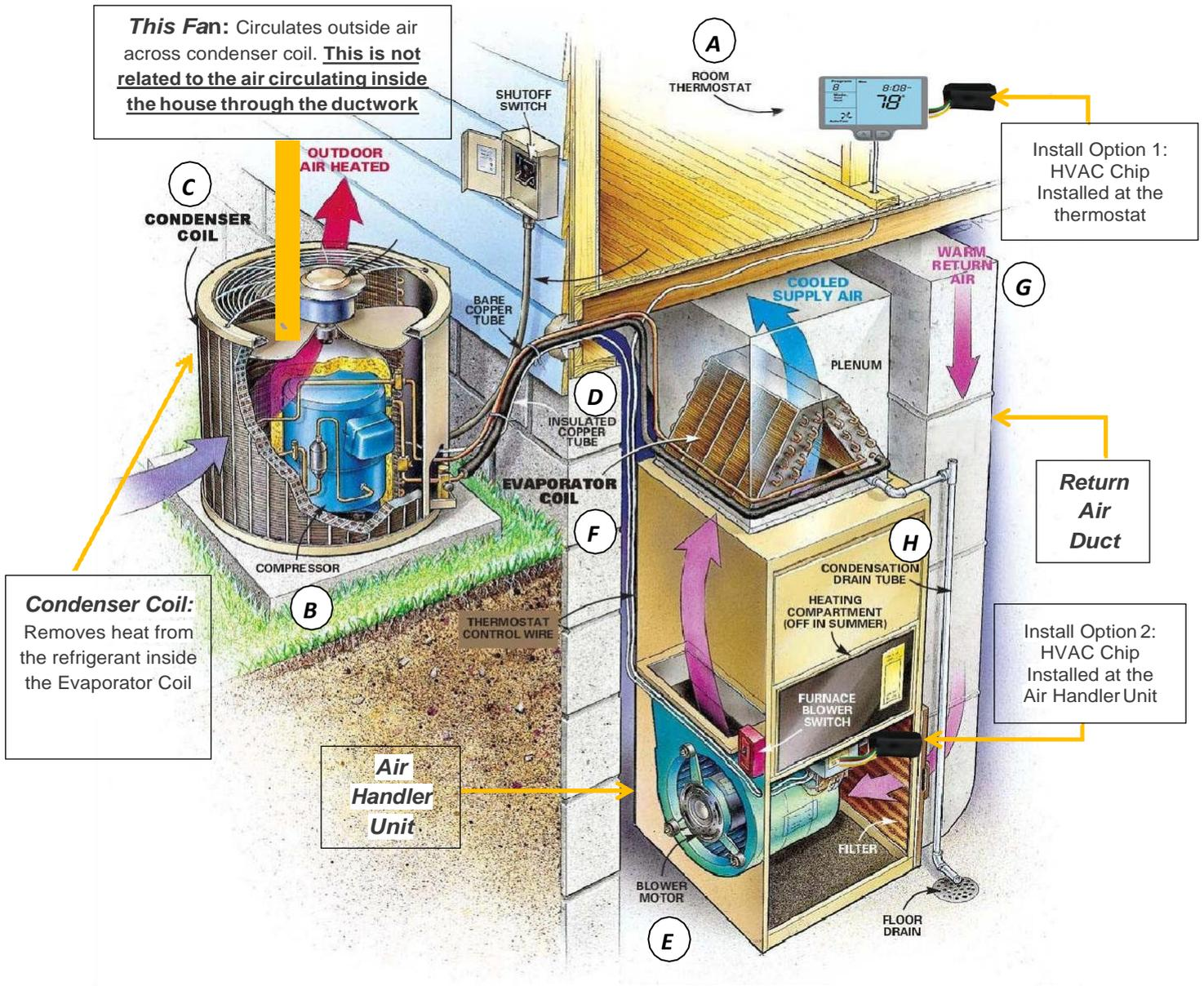
The above picture shows a typical HVAC system used in the United States, Canada, Mexico and other parts of the world where a central **Room Thermostat (A)** - top right in picture above) is used to detect the room air temperature and turn the HVAC system based on temperature settings.
