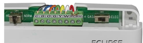
**WARNING: HP/NORM switch must select NORM for ELEC/GAS to operate**
