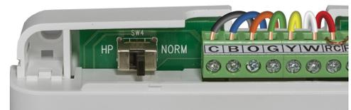
14. If the **NORM** is selected, then **ELEC/GAS** switch located at the right of the terminal block must be set to the corresponding heating energy source. For electric heating, select **ELEC**. For gas furnace heater, select **GAS**.
