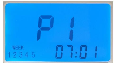
33. Continue to press “**SET SCHEDULE**” to set P2 for period 2 and so on, until all the 6 periods have been programmed. To turn off any period, press the “**SET SCHEDULE**” to the period (for example P1) and continue pressing “**SET SCHEDULE**” until the temperature set point is displayed. Then, press the **DOWN** button to lower the temperature until it displays **OFF**. This turns off the programming for that period (for example P1). This completes the programming for Monday to Friday.
