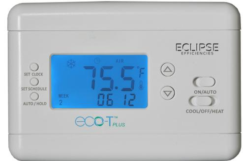
18. When the thermostat is set to **COOL**, the screen displays a **SNOWFLAKE** symbol in the top-left quadrant of the screen to indicate that the AC compressor is running. If this **SNOWFLAKE** symbol is flashing, the thermostat is on compressor short cycle delay. The compressor short cycle delay protects the compressor from **SHORT CYCLING**. This feature will not allow the compressor to turn on for 5 minutes after it was last turned off.
