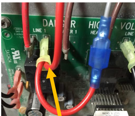
Photo 30. Connecting the insulated female connector of Cable 7 to Line 1 Terminal of PTAC system board.
