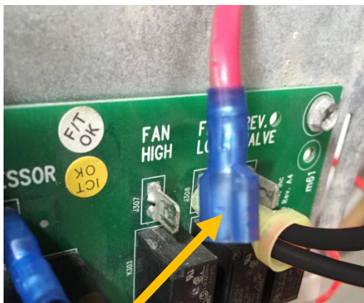
Photo 14: Adding the Insulated female connector
