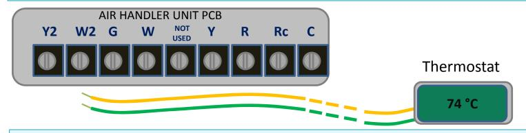
Step 4: Connect HVAC-Chip's **GRAY** WIRE to the thermostat's **GREEN** wire. *Note that the chip's gray and yellow wires must connect to the wires going to the thermostat.* Then, connect HVAC-Chip's **GREEN** WIRE to the "G" Terminal and the **PURPLE** wire to the "Y". *Note that the chip's green and purple wires must connect to the HVAC controller or to the fan and compressor wires going to the HVAC system.*
