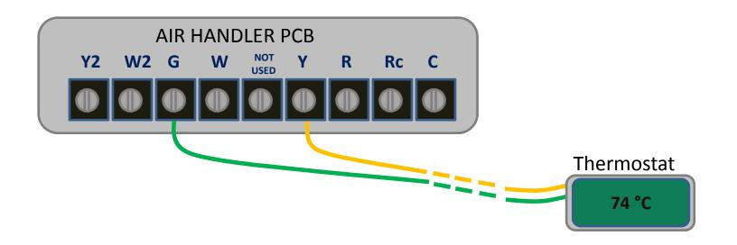
Step 3: Disconnect the **Green** wire from the "G" terminal and the **YELLOW** wire form the "Y" Terminal of the terminal block as shown below
