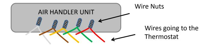
Step 2: Find the green and yellow wires. Remove the wire nut and separate the wires. *Then, identify which wires go to the thermostat and which wires go to the HVAC controller.* Tag the wires correctly.
