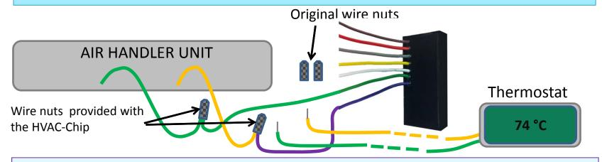
Step 4: Connect HVAC-Chip's **GRAY** WIRE to the **Green** wire going to the thermostat using the original wire nut and the Chip's **Yellow** to the **Yellow** wire going to the thermostat using the original wire nut as shown below. Note that the chip's gray and yellow wires must connect to the wires going to the thermostat.
