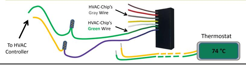
Basic Concept: Regardless of where at the Air Handler Unit the CWS-8THEM-0006 HVAC-Chip is installed, the **GREEN** and the **PURPLE** wires of this HVAC-Chip respectively always connect to the Fan and Compressor wires going to the HVAC system or HVAC controller. (See above picture)
