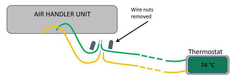
Step 3: Connect the **Green** wire of the HVAC-CHIP to the **Green** HVAC fan wire and the **Purple** wire of the HVAC-CHIP to the **Yellow** wire of the HVAC or Air Handler Unit as shown below.
